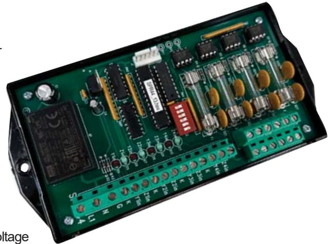
The SPR-44B operates over the standard SSI wide voltage range. The SPR-44B has a built-in low voltage transformer-isolated power supply generating a +13VDC wetting voltage
